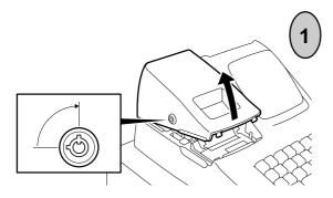
To remove the Printer Cover, insert the Printer Cover/Drawer key to the Printer Cover Lock, and then turn it 90° clockwise.
